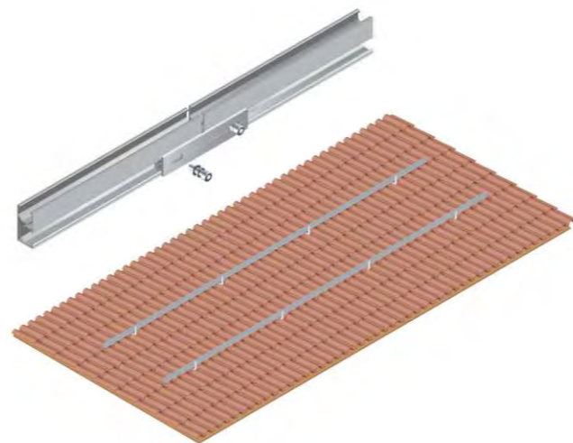
Step 4: Secure the rail on the hooks
