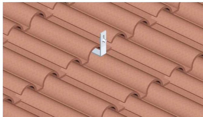
Step 2: Re-instate the Tiles
